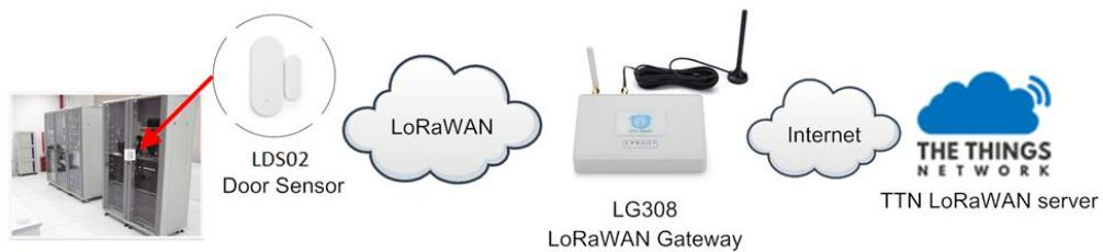
The LDS02 is installed on the door edge to detect the open / close event. And send the status to LoRaWAN server. The LDS02 will uplink two type of messages to the server.
